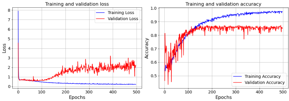
Figure 14. Train and validation loss and accuracy for the extended neural network model with feature attention, multi-head attention, and cross-network integration (500 epochs).
